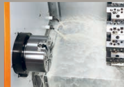
Coolant flush onto covers (Photo with opt. pump Grundos MTH4-40/4)
